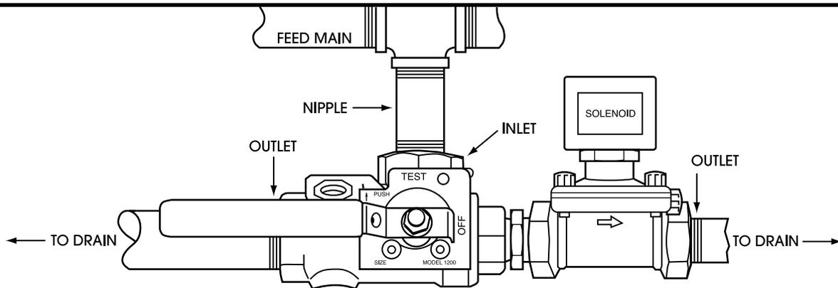
1. Check the indicating plate for the correct orifice size.  $\frac{3}{8}$ ",  $\frac{7}{16}$ ",  $\frac{1}{2}$ ",  $\frac{17}{32}$ ",  $\frac{5}{8}$ ", (ELO),  $\frac{3}{4}$ ", (ESFR).
